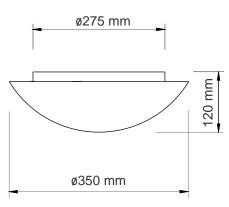
Protection degree:IP 43Diffuser:UV stabilized plasticLampshade colour:whitePower supply:230V 50HzLamp:2 x 23W / E27Body:steelFinishing of body:white powder coated
